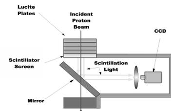
Fig. 1: Schematic view of CCD beam imaging system
