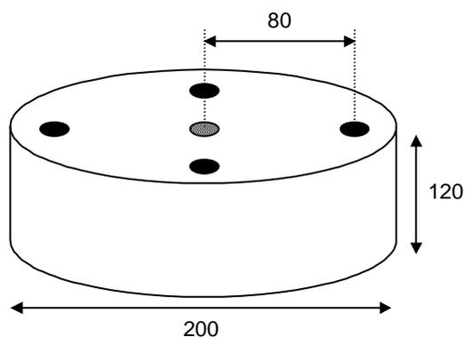
Figure 1: Scheme of the cylindrical PMMA phantom. The Ir-192 HDR source is located in the center hole. Holes indicated in black are for the thimble chamber. Dimensions are given in millimeters. The measuring depth and the source location are at phantom mid-depth.
