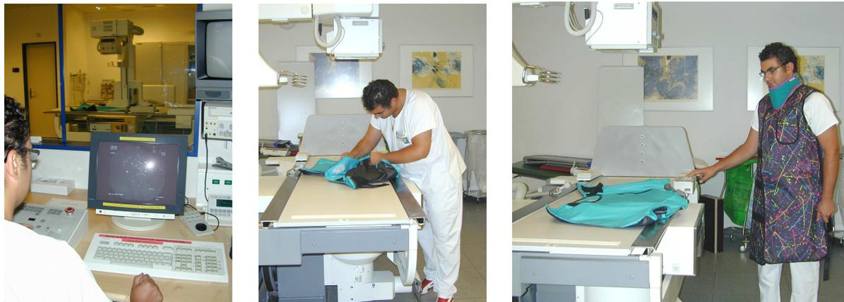
Figure 3: Testing X-Ray protection clothing using a fluoroscopy unit
