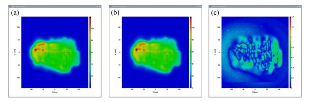
Fig. 2: Dose verification results for a large IMPT field (sacral chordoma case). (a) Calculated dose, (b) dose measured with CCD beam imaging system and (c)  $\gamma$ -Evaluation with  $\Delta D=3\%$  and  $\Delta d=3mm$  acceptance criteria for maximum dose and distance deviations.
